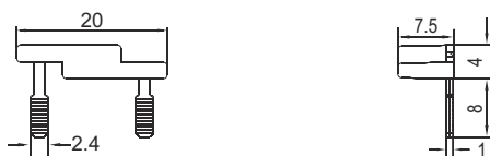
S1D-B1, 10A @ 250 VAC, 1 Way Bridge for Coil
