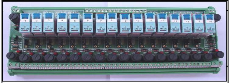
These Relay modules provide a compact, reliable & cost effective means of providing an isolation and safety barrier between the field equipment and the PLC
